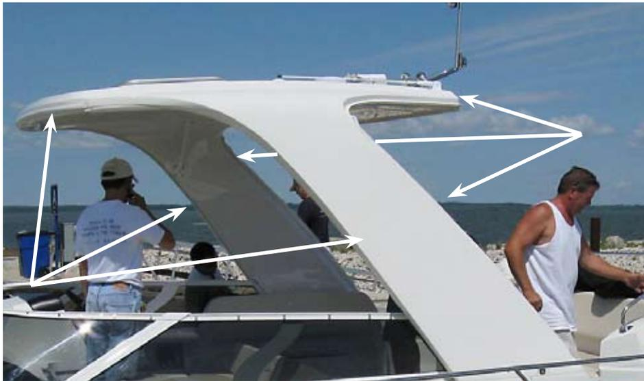
Slide into place the six pieces of sail track for the canvas top. Three in front and three in back . Pieces are marked. (top shown assembled).
