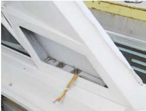
Pull wiring up from under seat access.
