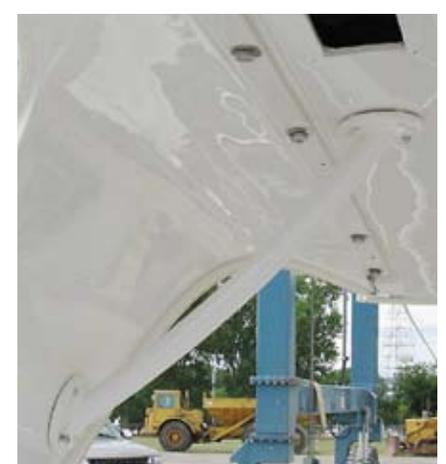
Check for port/stbd brace and install. Tighten screws.
