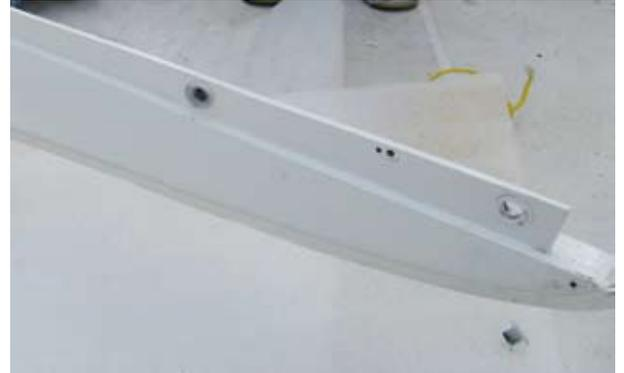
Replace plastic grommets in top of arch stubs with new ones supplied.
