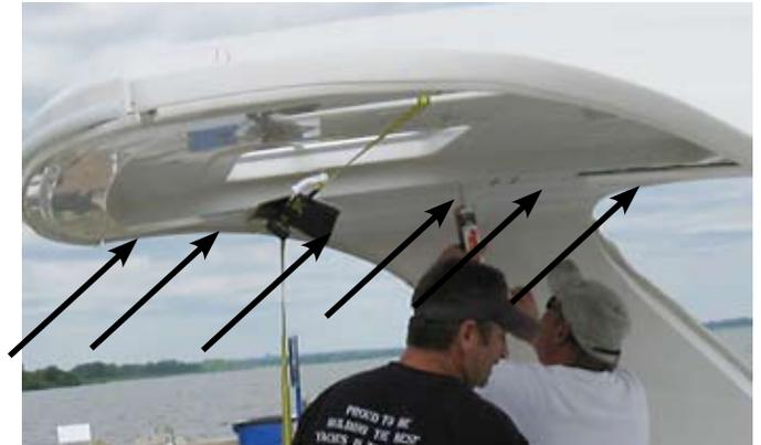
When lined up and in place, apply sealant on all bolts and tighten in place. Apply sealant to all seams inside and outside.
