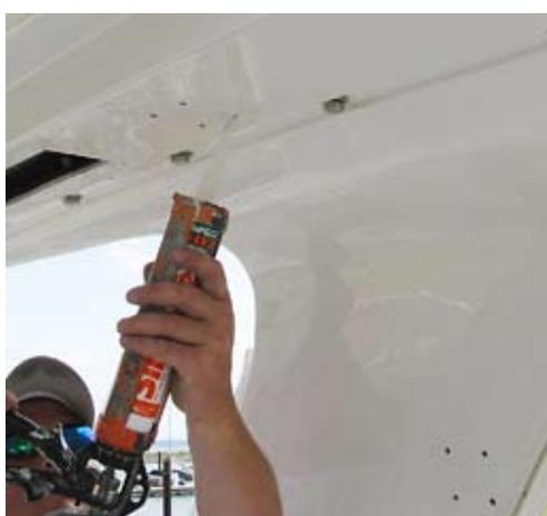
Clean area with acetone and apply sealant around mounting holes.
