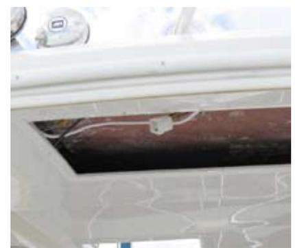
Connect wiring sockets in aft part of hardtop.
