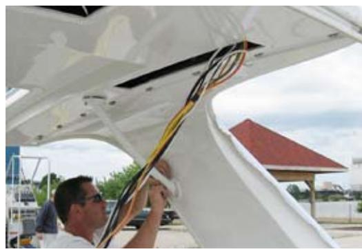
Pull wiring free from hardtop and feed down through arch stub.
