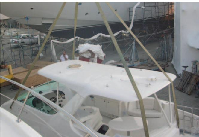
Bridge picking with crane. Use same pick points when picking with travel lift or forklift.
