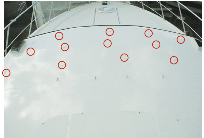
Cabin Top: Place dab of sealant forward of forward deck bolts.
