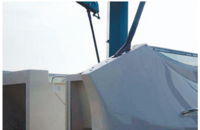
5. Run all wires up through the bridge aft port and starboard corners. Set the bridge in place, making sure that no wires are caught or pinched off. Make sure that the bridge is set with the alignment marks correct.
