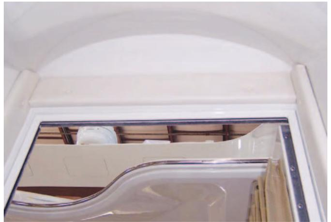
12. Install the navigation light and/or the radar pedestal being sure to use Tuff-Gel on all bolts and marine seal the wire hole into arch.
