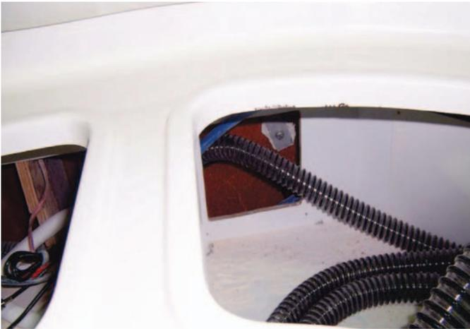
4. Apply sealant (732 white silicone # 8101201) around deck bolts. There are four bolts across the front and one in each aft corner.
